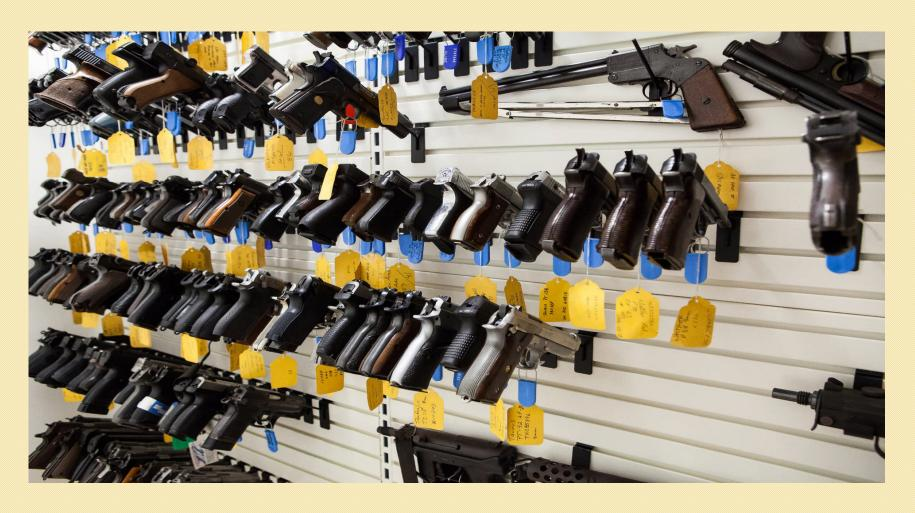
A portion of the firearms that comprise the Laboratory's reference collection; these are used to produce test fires during examination of evidence submitted for Firearms analysis.
