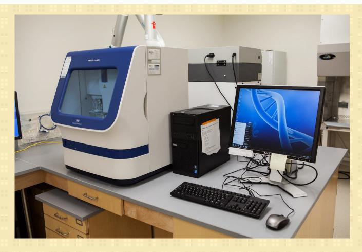
This is the instrument used to generate DNA profiles during analysis of evidence from criminal investigations or processing of convicted offender samples.
